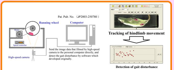
Feature O GAIT realizes automatic detection of gait disturbance in rats and mice, and is capable of quantifying it easily and precisely.
